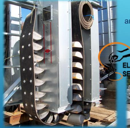
Productivity Q -1000 t/h., Lifting height along the axes of the drums no more H – 60m Bucket elevators type NCC are designed for vertical transportation of grain and other bulk products..
